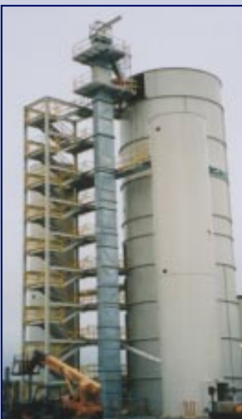
Six compartment aggregate storage bin - Bucket elevator - Cement storage silo
